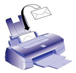
Set the thickness lever to the + position when you print on envelopes or if ink smears when you print on other thick media. Open the printer cover and position the lever as shown below. Then close the cover and print. (Make sure you return the lever to the 0 position before you print on thin media.)
